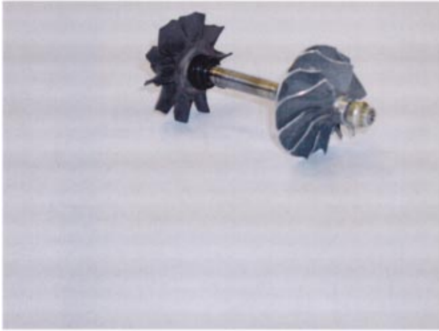
Fig. 8 Automobile turbocharger rotor (courtesy Honeywell)
