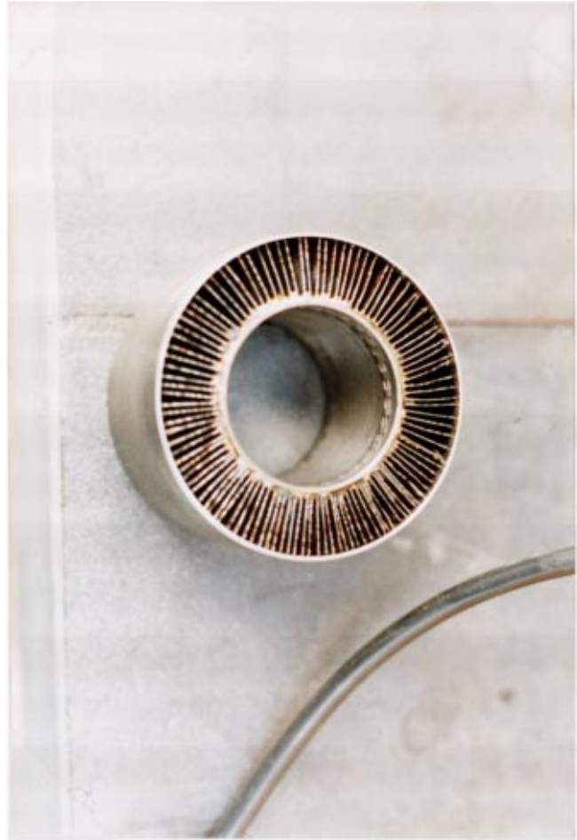
Fig. 9 Small primary-surface annular recuperator (courtesy Turbulence Tubes)
